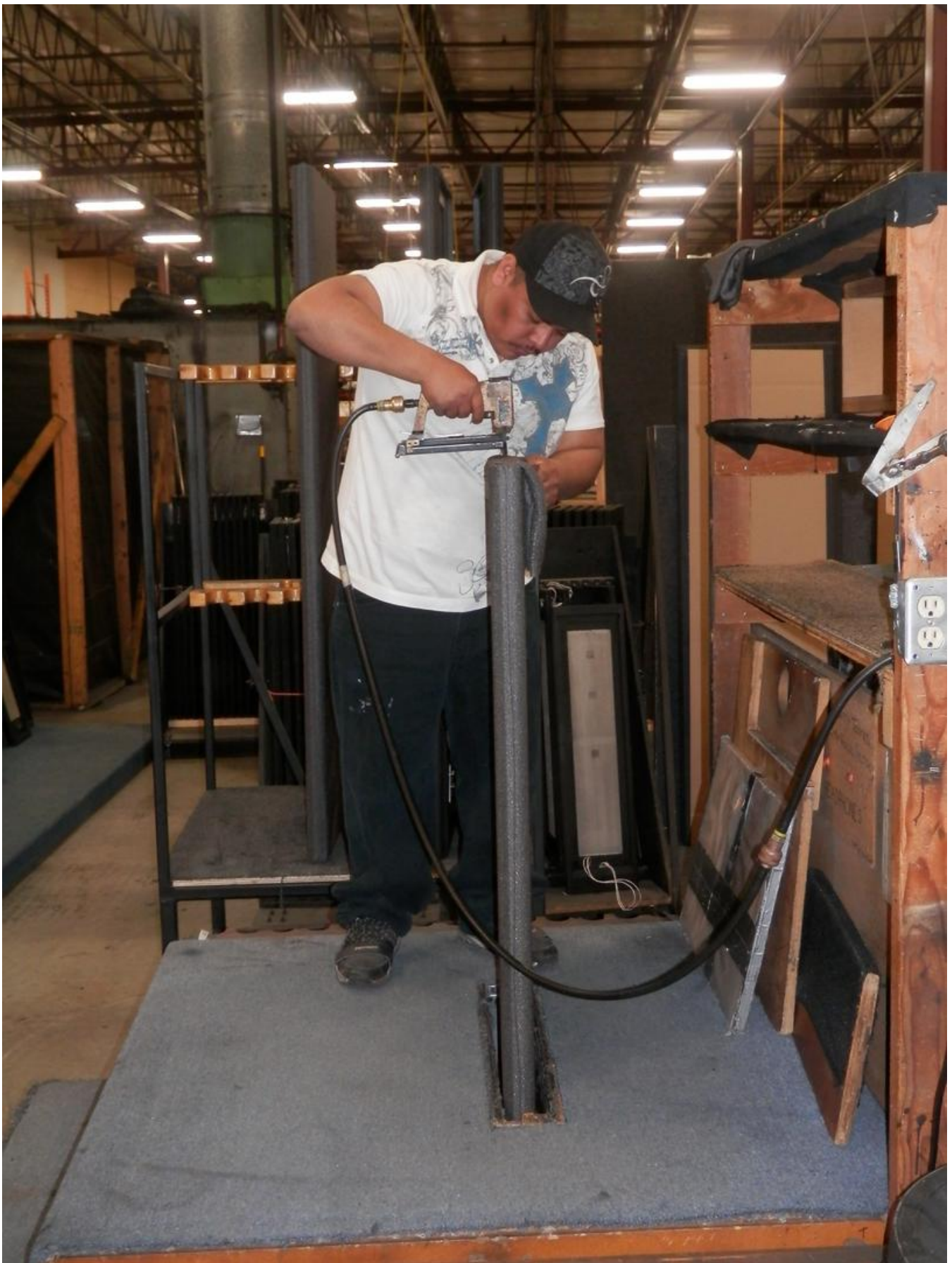
A technician fastens the grille “sock” to the bottom of a Magnepan’s frame.
