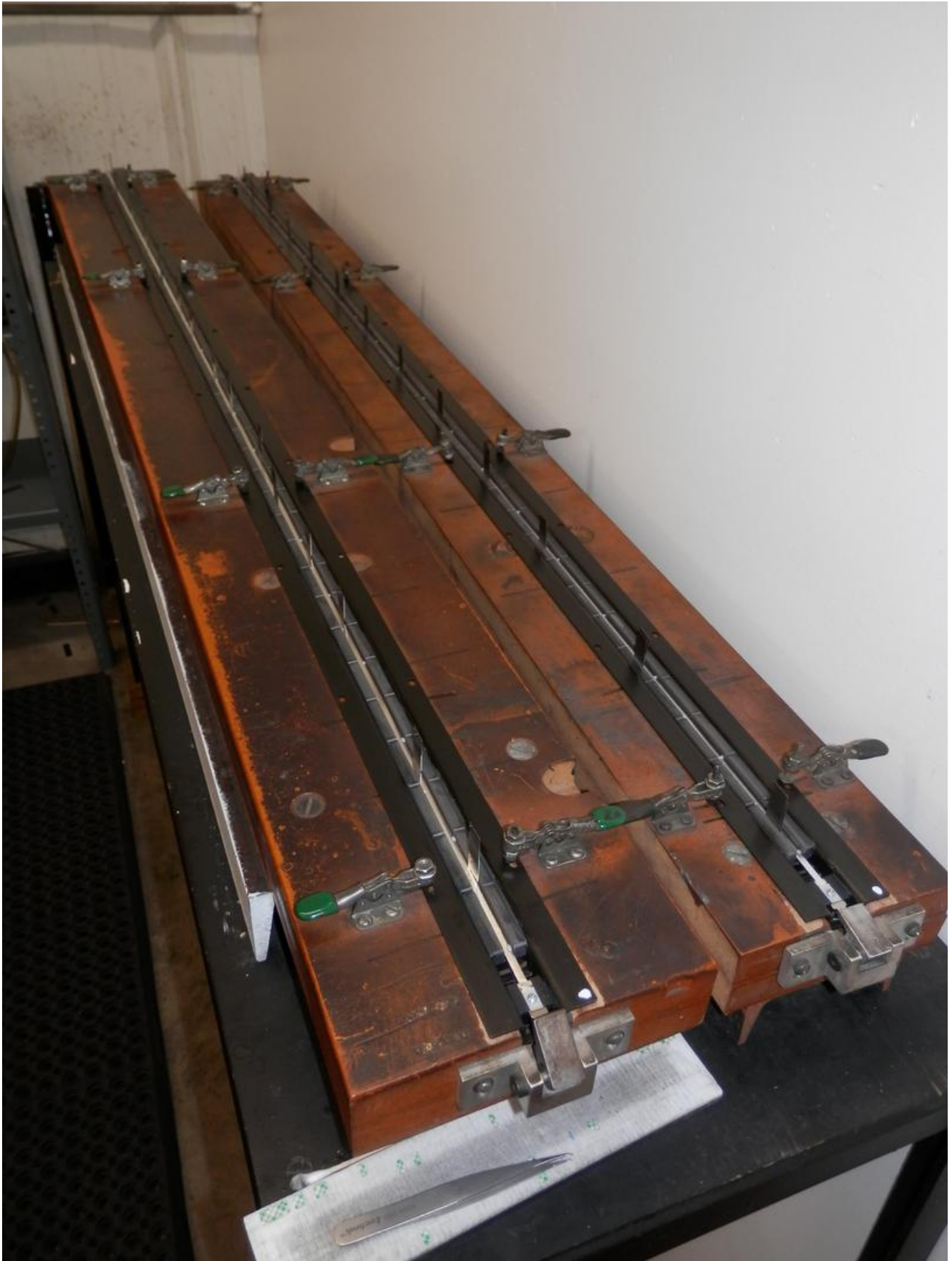
Tooling stands as used in building the ribbon tweeters for the Magnepan 20.7 and 3.7.
