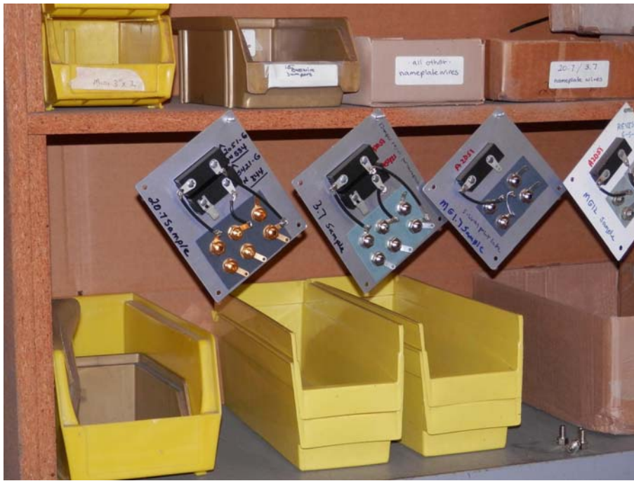
Samples of Magnepan terminal block assemblies as used for each of the firm's models.
