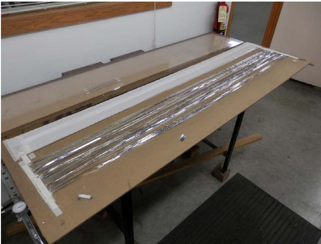
Ribbon diaphragms are pre-trimmed to the correct length.
