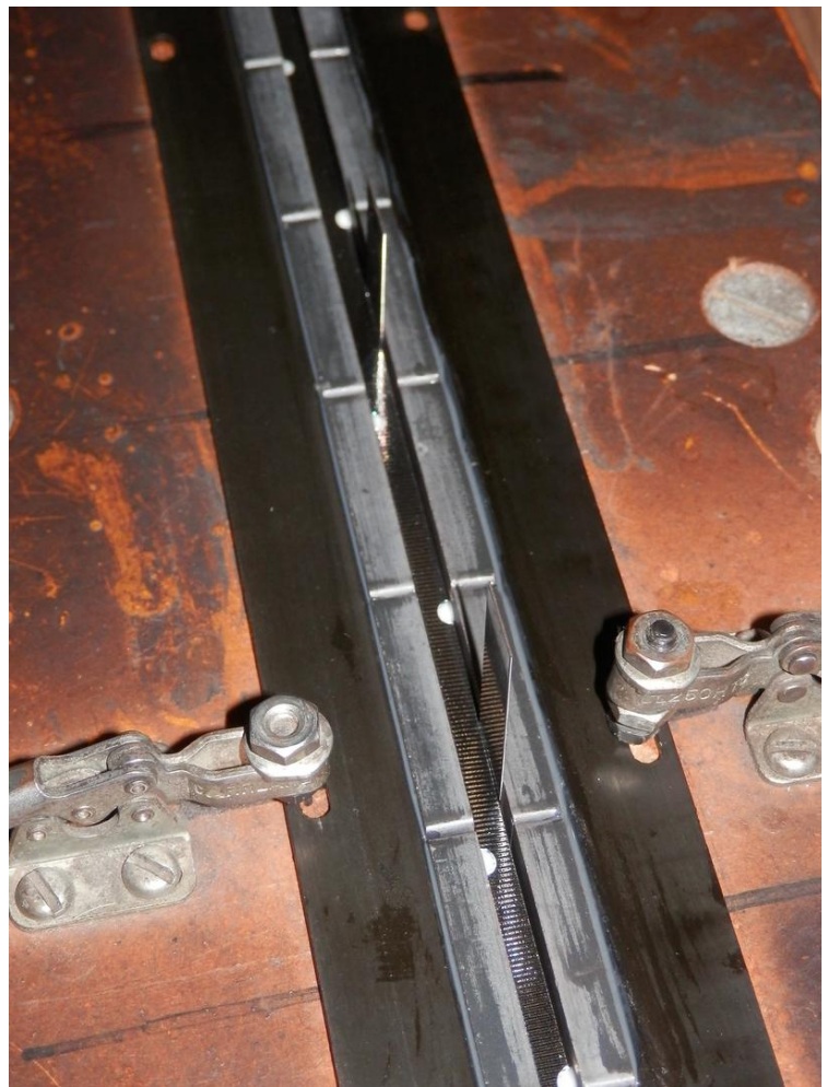
Ribbon diaphragms are pre-trimmed to the correct length.
