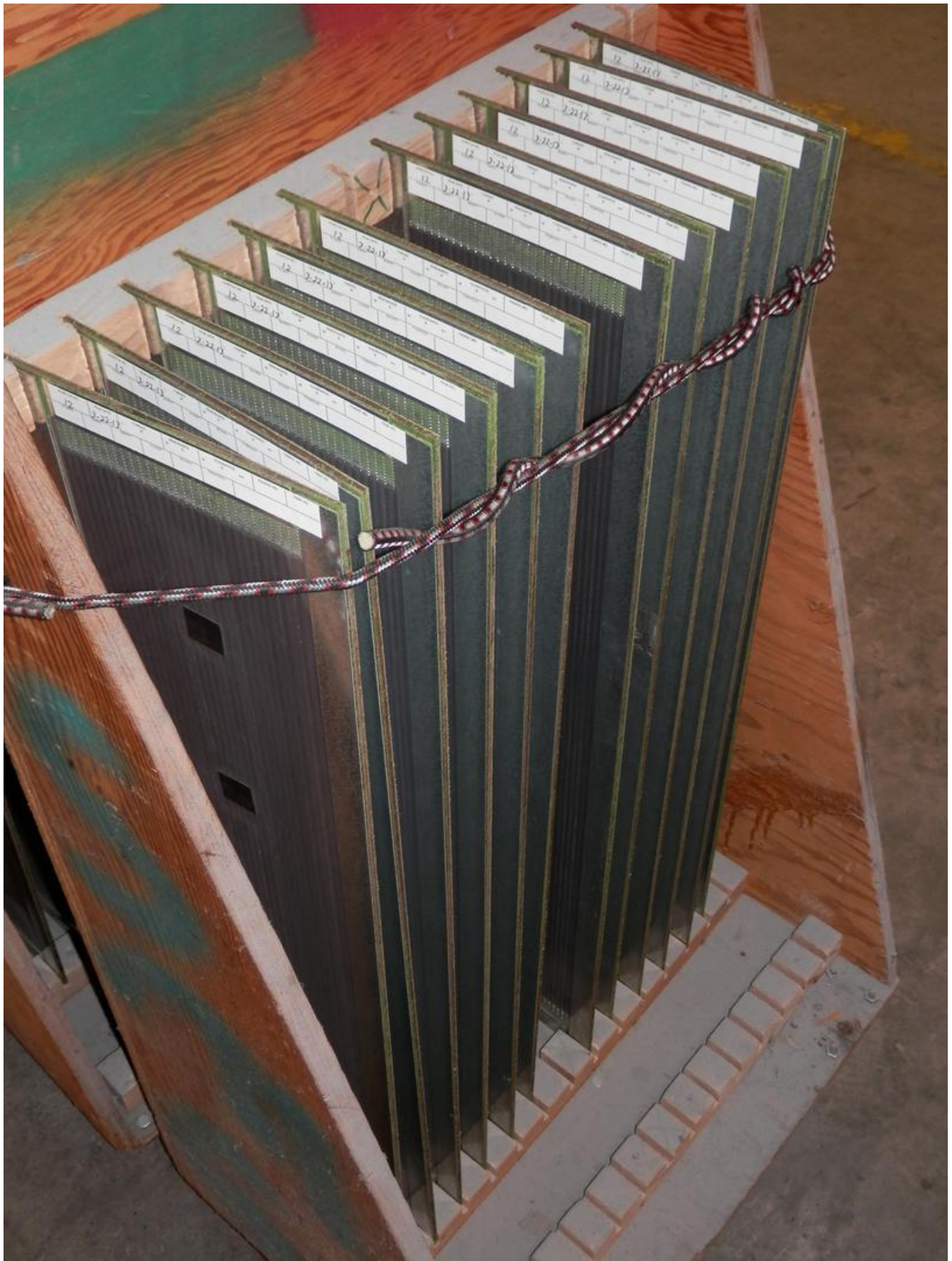
Sets of now Mylar-fitted driver assemblies await the next manufacturing step. Note that at this point each driver is marked with a sticker for tracking manufacturing steps.
